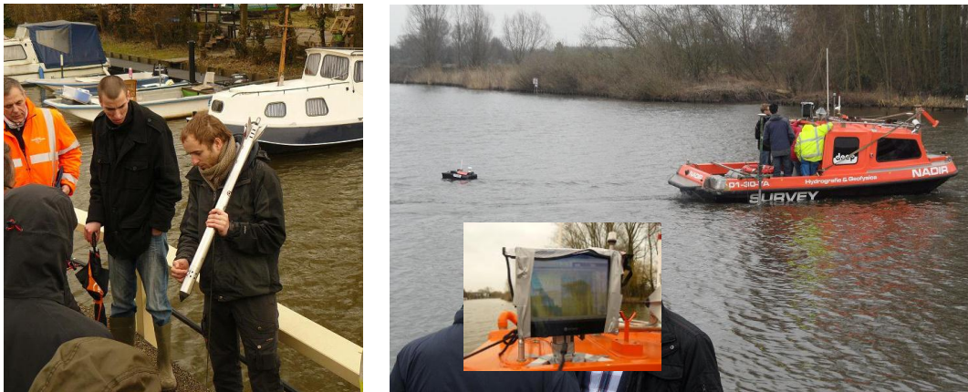
Links: dotOcean; GraviProbe. Rechts: Deep; boot met sub bottom profiler
